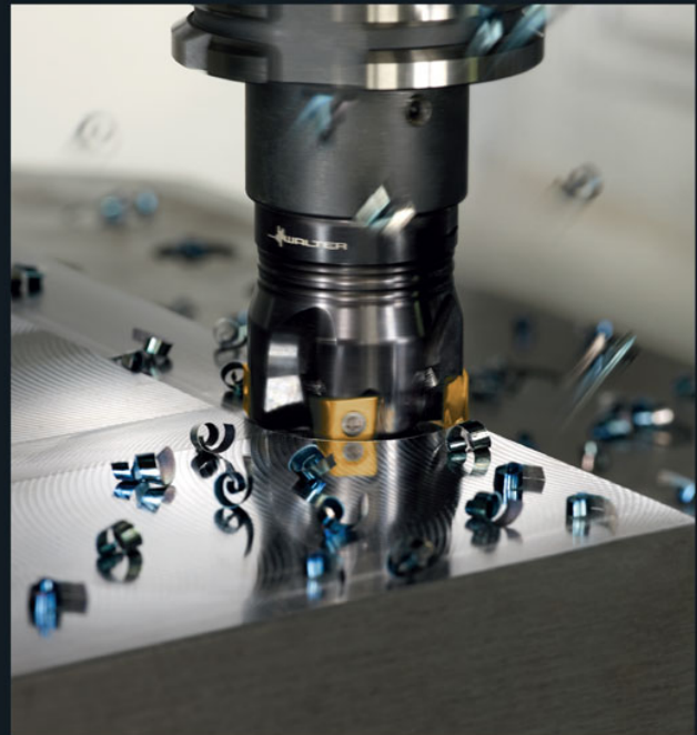
The Walter BLAXX F5041 shoulder milling cutter with Tiger-tec® Gold during machining. What is especially remarkable is that while field test results showed a tool life that was on average 80% longer, users in today's market report performance increases averaging between 100% and 200%.
